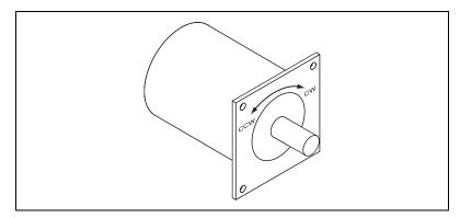
Figure 8. Clockwise and Counter-Clockwise Motor Rotation
